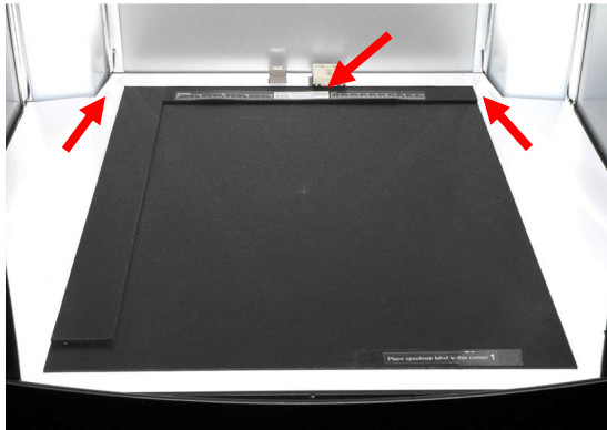
Figure 9. Proper position of specimen holder.
